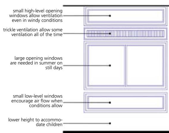
**Figure 18:** Ventilation options for varying conditions
