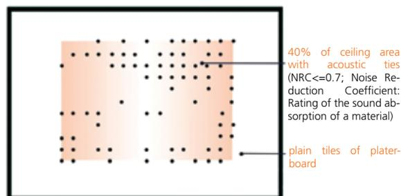
Figure 10: In new or existing classrooms with floor areas of 100 m<sup>2</sup> or less, covering 40% of the ceiling area with acoustic tiles is a low-cost and efficient option for noise reduction.
